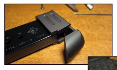
Slip on the power plate and screw it to the extension.
