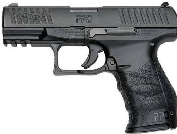
The PPQ has a terrific single action trigger mechanism, but the trigger take-up may feel a little sticky or gritty on some. However, it can be made to feel perfectly smooth. There are several areas that could cause some gritty feedback, but it will most likely be the result of the safety plunger operation, that is, the action of the trigger bar ear as it passes over and depresses the safety plunger.
