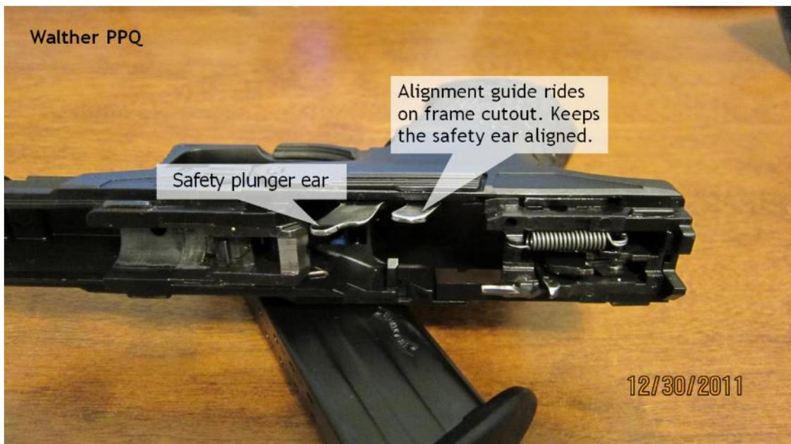
With the slide mounted, you can look down into the grip and see the action of the ear on the safety plunger. You can work the trigger and see the plunger in action. In my case, the ear was not aligned to the center of the safety plunger's ramp and was riding towards the outer edge. I could also feel the grittiness as well as get visual feedback while working the trigger, so it was pretty clear this was on the right track.
