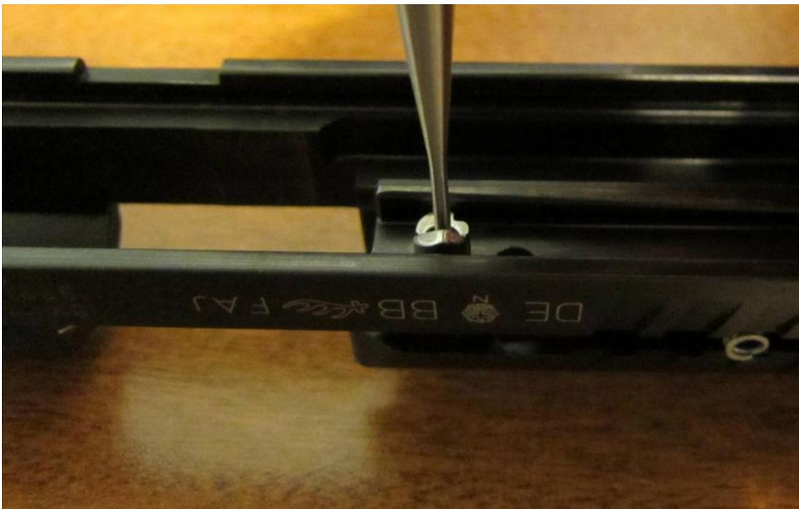
Next, I gently depressed the plunger at various angles, and felt the same grittiness as when working the trigger. It was pretty obvious the plunger needed to be depressed as vertically as possible. The ramp was going to add enough side forces as is, so having the ear ride center to it, or even erring slightly to inboard, would be necessary.
