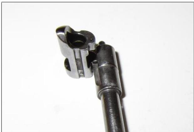
**This represents the plunger depressed, allowing the striker to pass and fully extend.**
